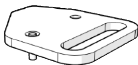
Figure 62 - Flywheel locking tool
